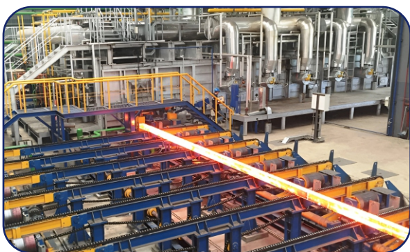
SKID TRANSFER MECHANISM
